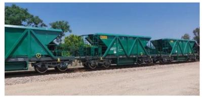
Hopper wagon acquired for the installation of Variable Gauge Axle (EAVM)
