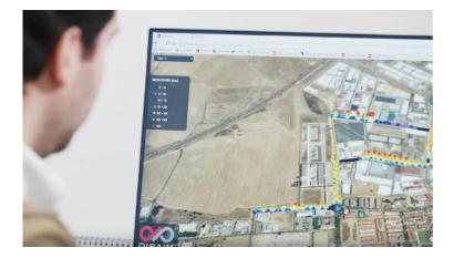
The project undertaken by **REISSWOLF SUROESTE S.L.** consisted of a cloud computing tool to optimise the management of its vehicle fleet, safety and metrics collection. The solution makes it possible to configure alerts, routes and different productivity measures, including variables such as speed control, the number of operating hours and telecommunications cost control.
