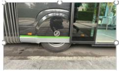
Wheel arch fairing to improve aerodynamics and energy efficiency
